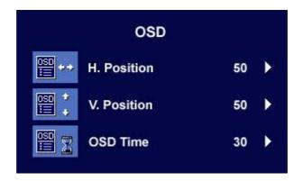
Press the or keys to adjust the **Horizontal Position** of the OSD.
